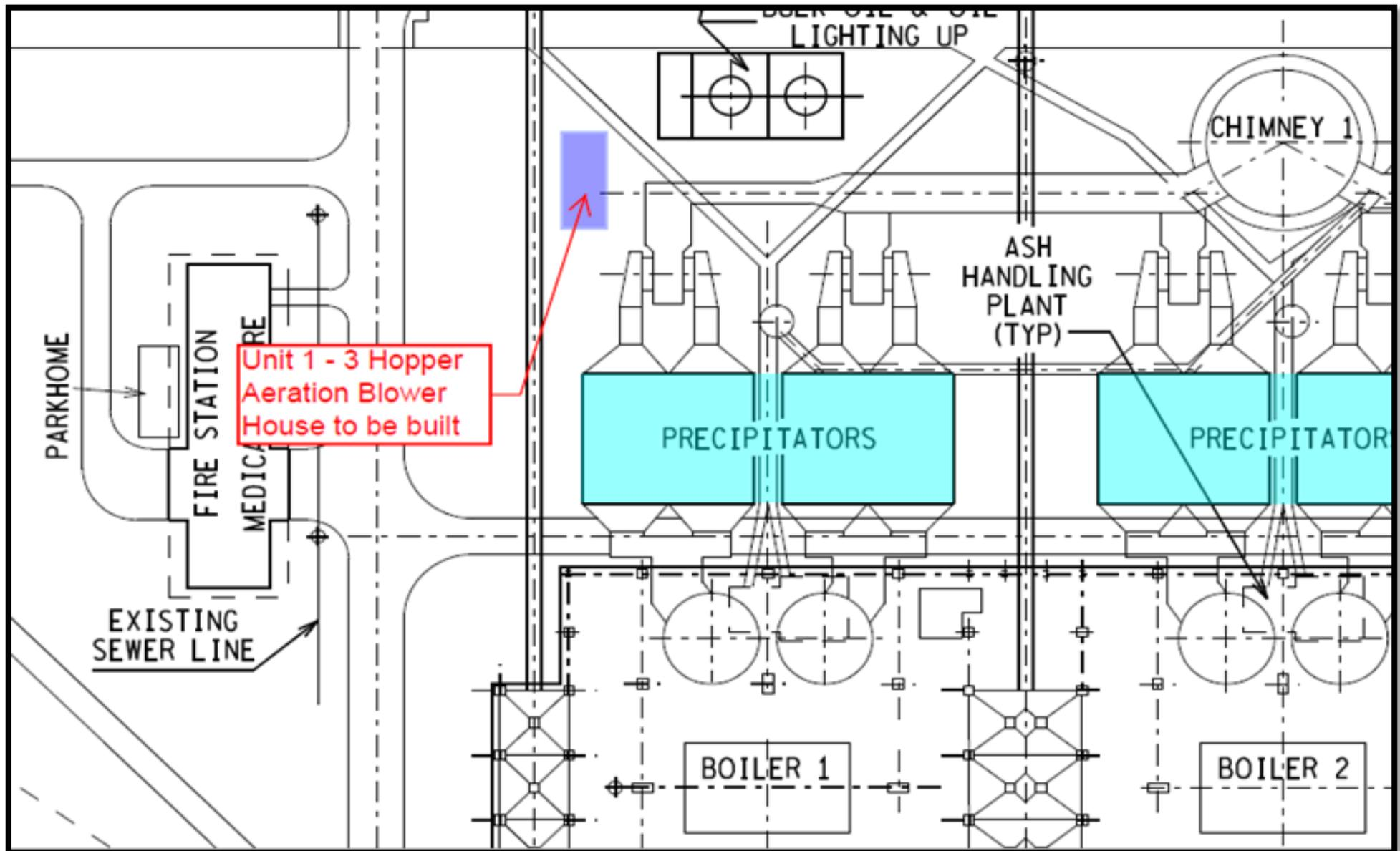
Figure 3: Position of the Blower House for the Aeration System
