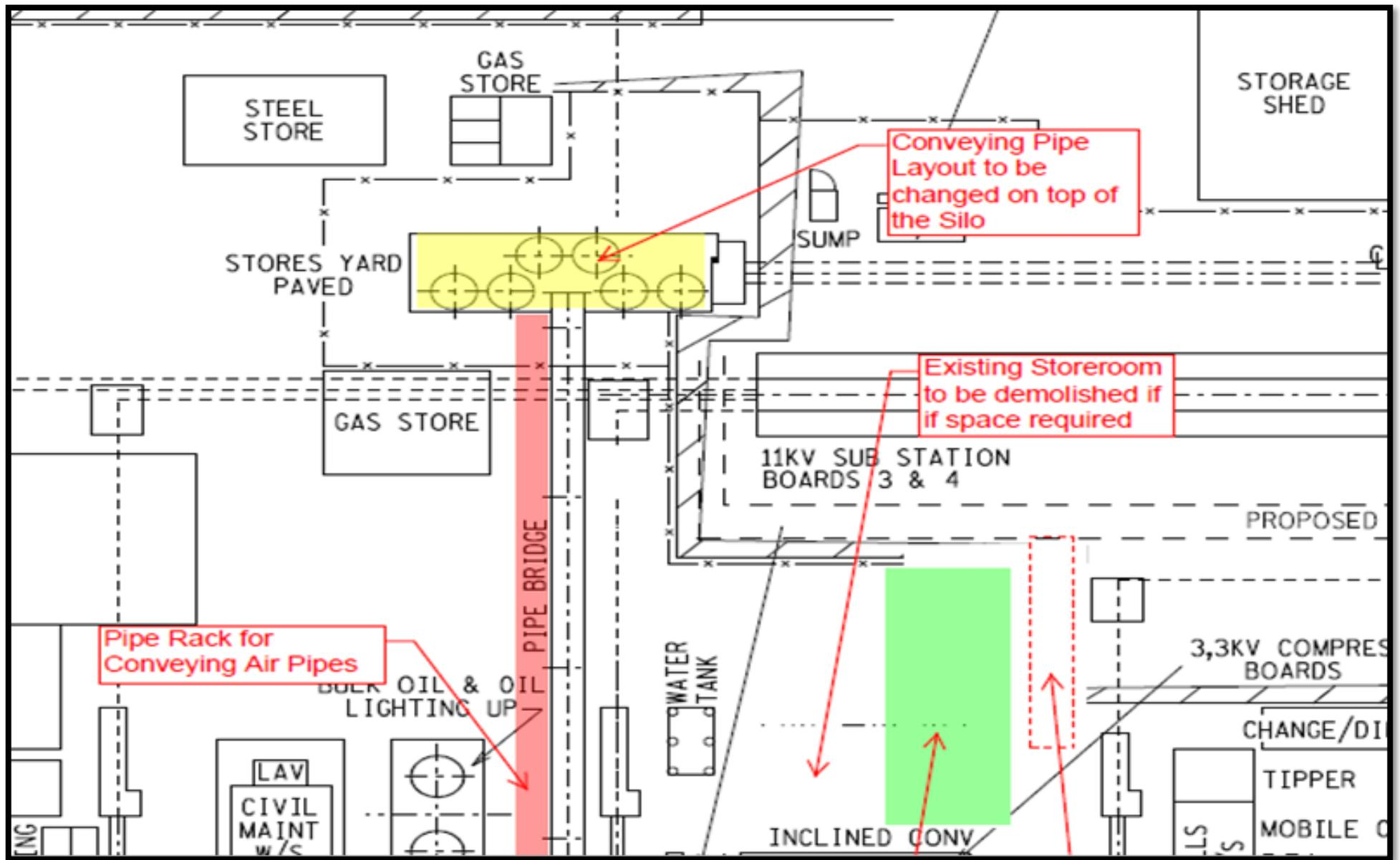
Figure 1: Layout of Upgraded DHP with Chain Conveyors and Bucket Elevator Technology for Two Units
