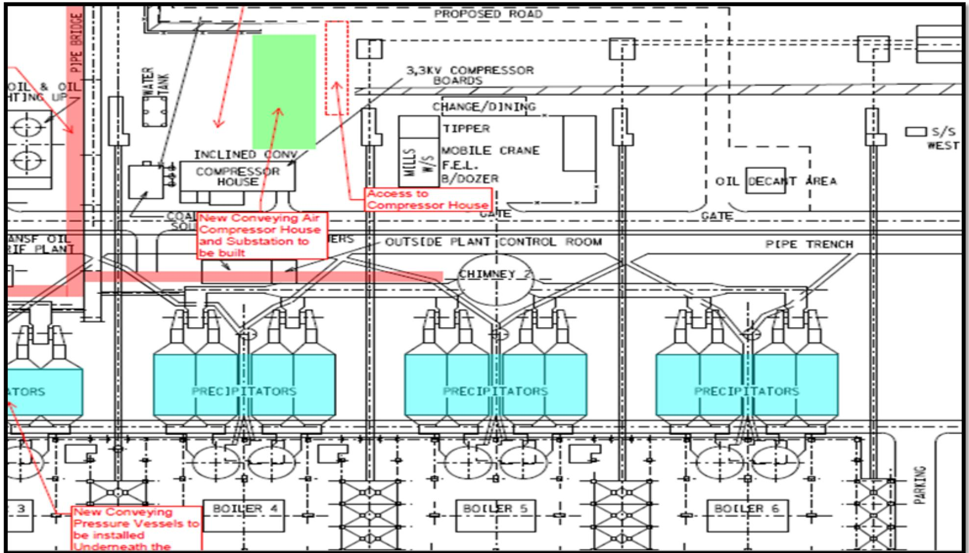
Figure 2: Position of the Compressor House for the Pneumatic DHP
